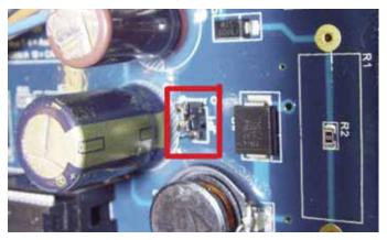
To reset the display to go ON with the ignition, disconnect and remove the display from the vehicle, open the case, remove the jumper and place over BOTH pins - see photograph 3.
