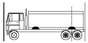
4b - 4 load cell system. 1 off - 6 way junction box and inclinometer.
