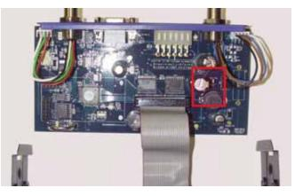
A close up view - see photo 2 - shows the jumper located only on one of the pins, for storage.
